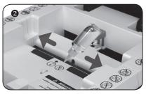
3. Close lid and turn shredder in reverse mode for 3-5 seconds.
