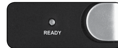
Ready (Power On)
