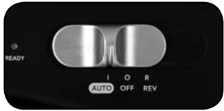
▲ Power switch in auto position
