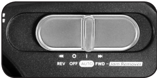
▲ Power switch in auto position
